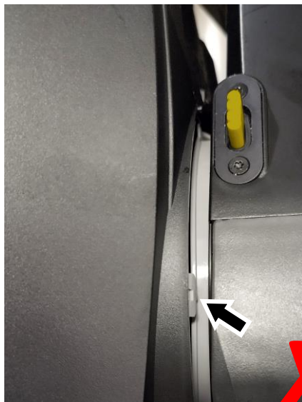
Incorrect – tab outside head cover
